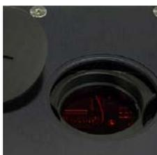
High-performance servo motors featuring rare Earth magnets coupled with backlash-free power transfer provide ultimate torque which translates to ultimate speed. Adjacent filter distance is traveled in 30ms while the longest distance (5 filter positions or 180 degree wheel turn) is covered in less than 100ms. An additional benefit of servo motors is the use of encoder feedback
