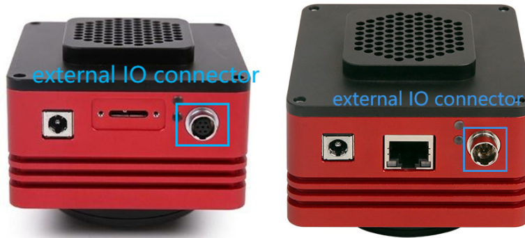
Figure 38 SWIR series side appearance information
