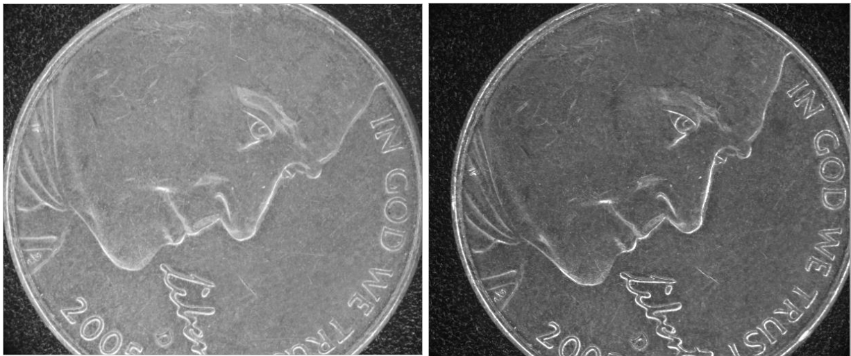
Figure 5-54 Ordinary camera (left) compared with polarizing camera (right) metal surface effect
