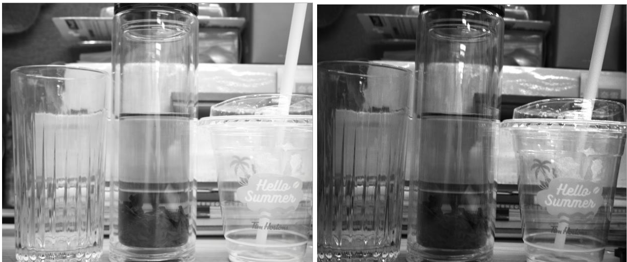
Figure 5-52 Comparison of plastic surface effects between ordinary camera (left) and polarizing camera (right)
