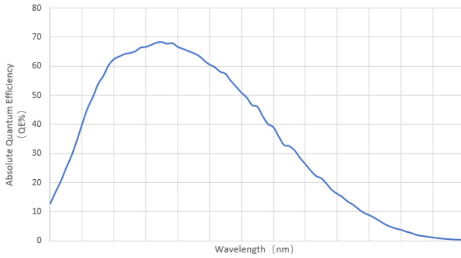
Figure 5-37 SC273M-ICM absolute quantum efficiency
